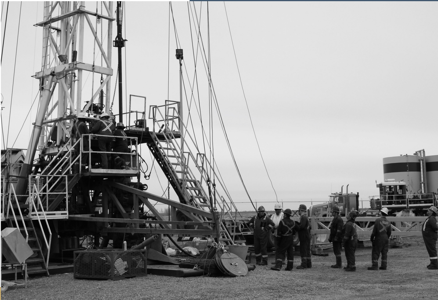
The drilling rig established to pull and replace the injection well tubing in May, 2018
