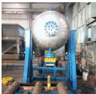
The physical model at the Saskatchewan Research Council's Energy Division remains a key tool for modeling oil reservoirs.
