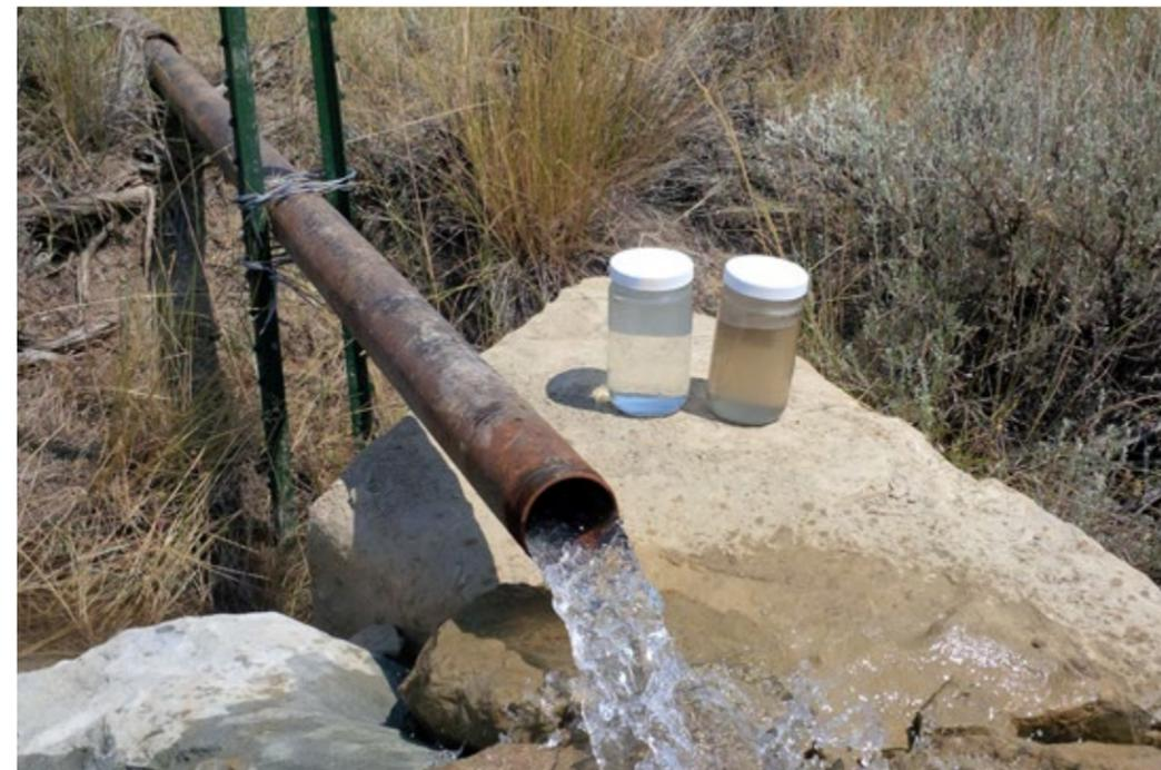
*Untreated water in the right glass container, with treated water on the left. The pipe shows full production of treated water from the ERIN field trials.*
