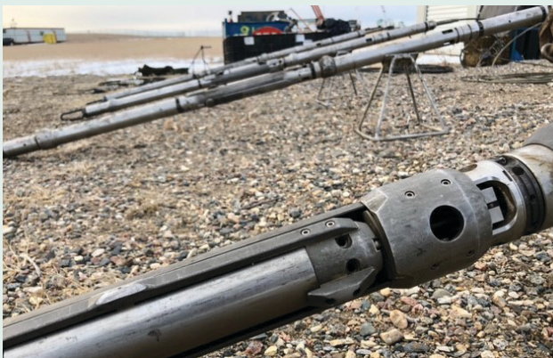
Crosswell geophones about to be deployed.
